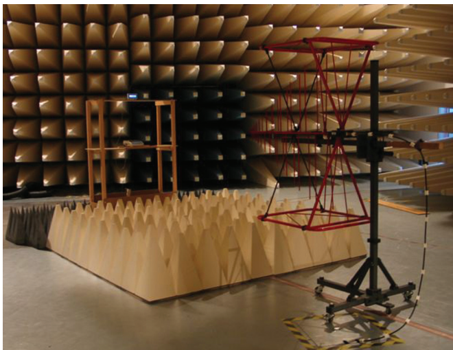
Anechoic chamber used for electromagnetic compatibility (EMC) testing.
