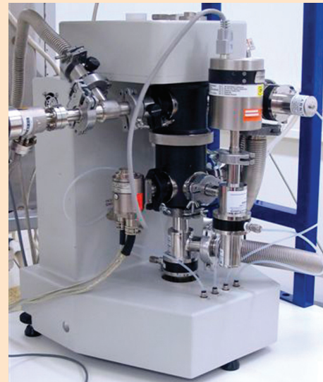
Primary vacuum standard based on conical piston technology.
